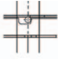
B. UltraBAR™ JOINT SYSTEM IS SECURE AND PROTECTED FROM VANDALISM BY INNER AND OUTER RAILS
